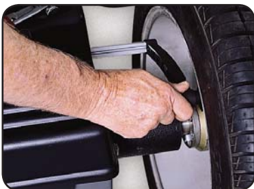
Inner geodata arm measures wheel distance and diameter
