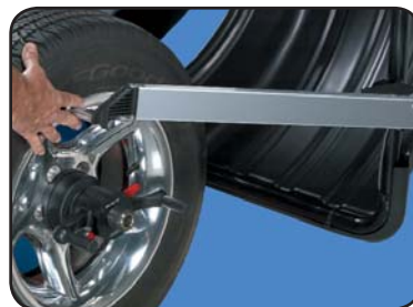
Outer geodata arm measures wheel width
