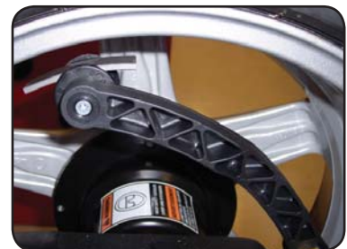
Inner geodata arm also places tape weights behind spokes or on inner edge of wheel
